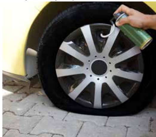
Sealant injected through the tyre valve
