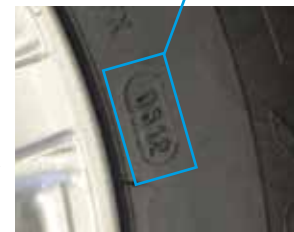
The DOT 1 number indicates the week and year the tyre was manufactured
