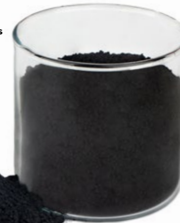
Binding agents and pigments Carbon black from pyrolysis becomes a new raw material to act as a binding agent or pigment, etc.
